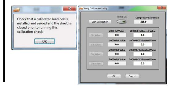
There will be a series of four tests at increasing values. The left column displays the amount of pressure that the CLF-40 pressure sensor is reading. The column on the right is blank until the reading from the external load cell is entered manually.
